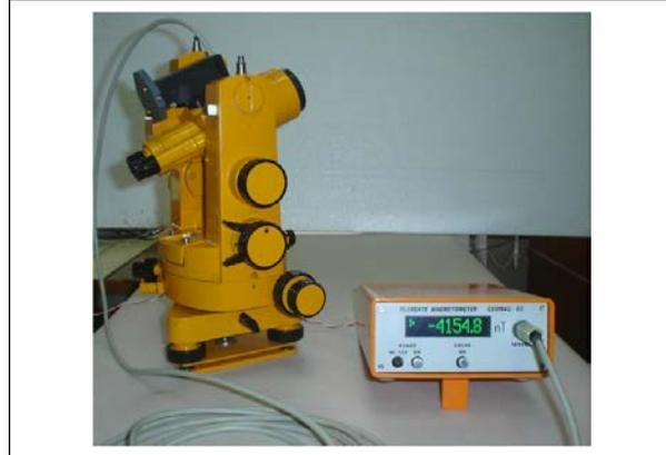
Inclinometer/declinometer installed in non-magnetic theodolite
